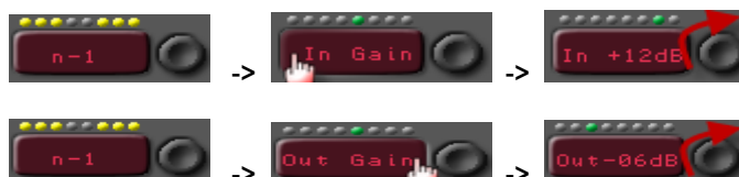
Figure 466: Operating “Set In/Output Gain” on the panel (direct access)
