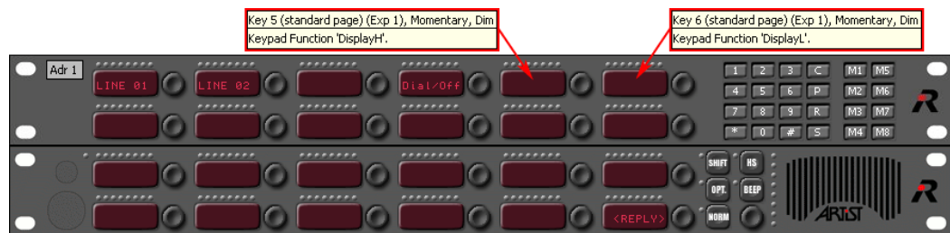
Figure 531: Connect - Keypad panel setup
