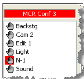
Figure 610: MCR handling - Active audio in a conference. Source is "N-1"
