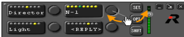
Figure 376: VCP-10xx - Changing Volume on a VCP-1004
