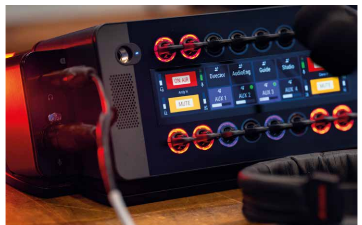
Commentary Control App with Commentary Headset Adapter providing 2 × XLR-3F and 6.35 mm stereo jack connectivity
