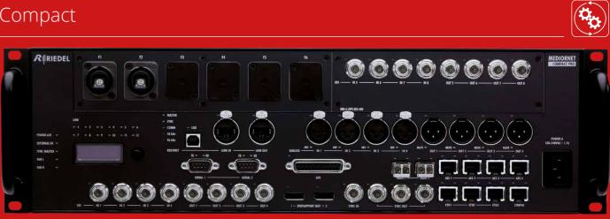
MediorNet Compact is the cost-effective and easy-to-use entry to the world of MediorNet. With a network bandwidth of 50 Gbit/s, MediorNet Compact provides enough capacity for bi-directional transport of 16 HD-SDI signal, dozens of MADI streams or GBit-Ethernet signals and hundreds of audio channels or intercom ports.
